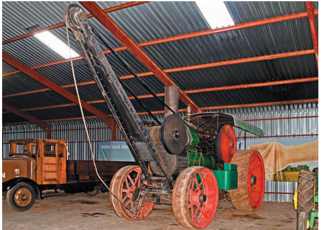
Fowler B5 crane locomotive of 1901.
