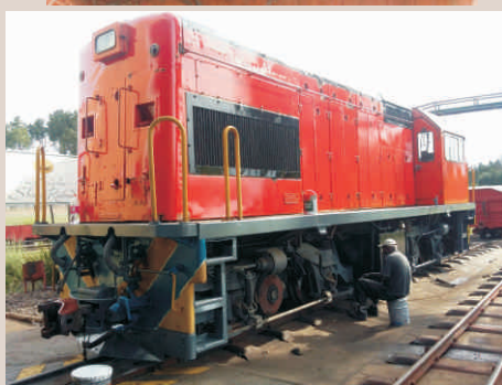
Left & above, once safely in the Sandstone depot, the maintenance team immediately commenced cleaning and repainting the Class 91 in Spoornet orange
